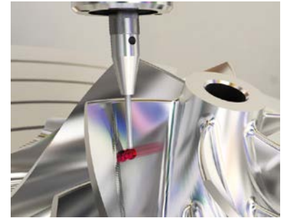
Scanning procedure for checking of workpiece surface
